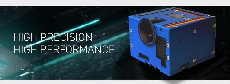
The iADCS400 is a fully autonomous attitude determination and control system aimed at small satellites with a 6U CubeSat form factor or a larger 12U form factor. It is based on the ST200 star tracker, complemented with RW400 series reaction wheels, MTQ400 series magnetorquers and features an optional external magnetometer, sun sensors, GNSS receivers or precision gyro. It can also host the CP400 Payload Processor inside to save the user additional space.
